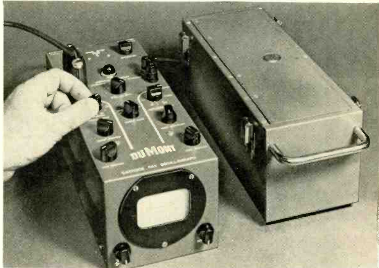
The transistorized oscillograph. The box at right holds the battery power supply.
