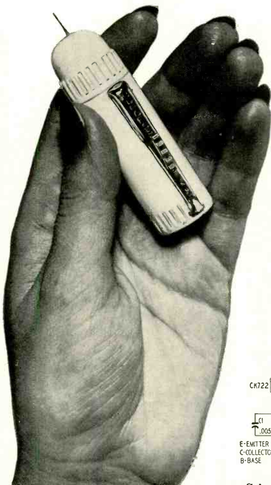
The completed signal injector.
