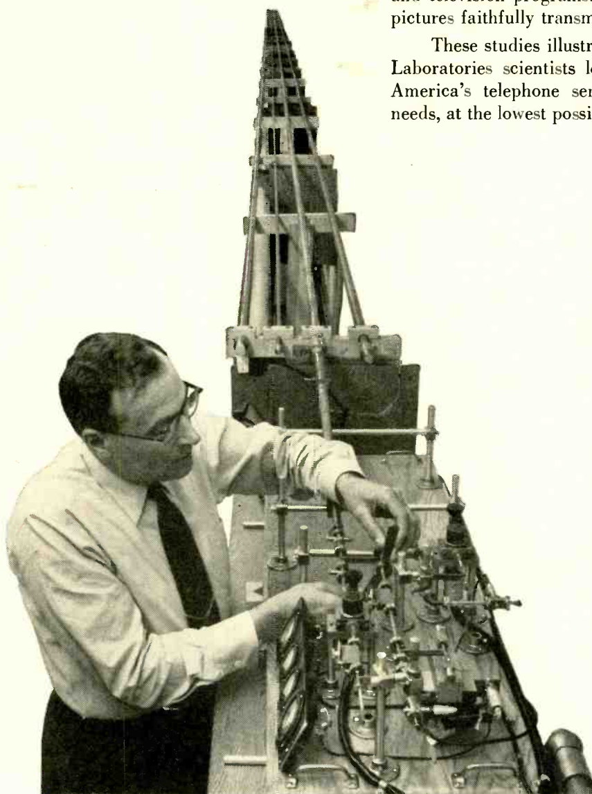
Testing round waveguides at Bell Telephone Laboratories, Holmdel, New Jersey. Unlike coaxial cable, waveguides have no central conductor. Theoretically, voice-capacity is much greater than in coaxial cable.
