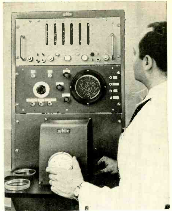
Du Mont's Iconumerator , a device which can count objects of any size and shape in its field of vision. Here its subjects are similar to colonies of bacteria counted in medical laboratories, etc. The most startling feature of the instrument is that the size of the object (as long as it can be contained in the field) or its shape make no difference in the accuracy of the numeration.
